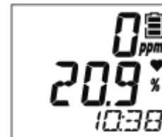
Upper row: CO (carbon monoxide) gas concentration display Middle row: O2 (oxygen) gas concentration display
